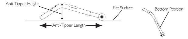
FIGURE 9.1 Installing/Adjusting Anti-tippers - Anti-Tipper Length
